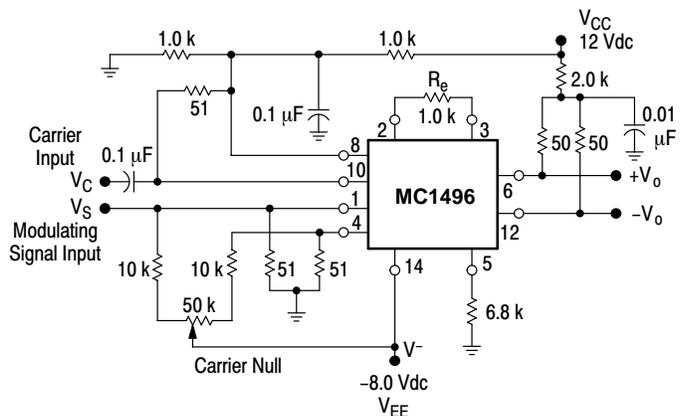
Figure 8. Transconductance Bandwidth
