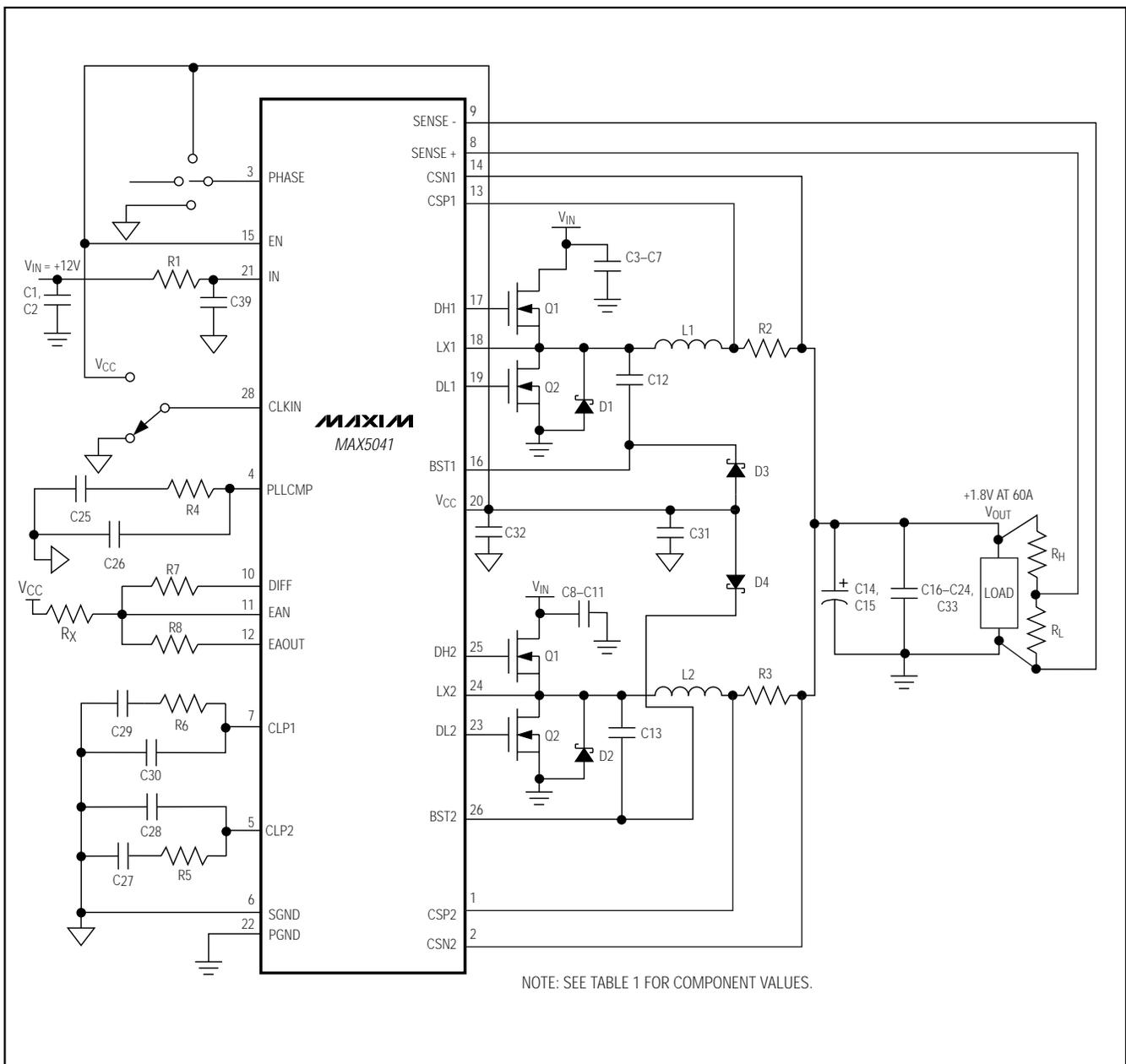
Figure 2. MAX5041 Typical Application Circuit,  $V_{IN} = +12V$
