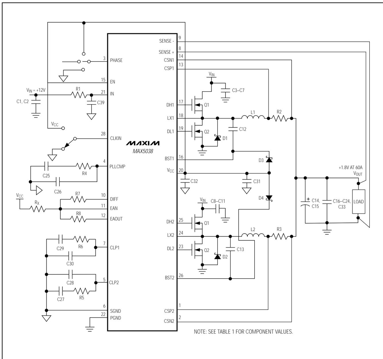
Figure 1. MAX5038 Typical Application Circuit,  $V_{IN} = +12V$
