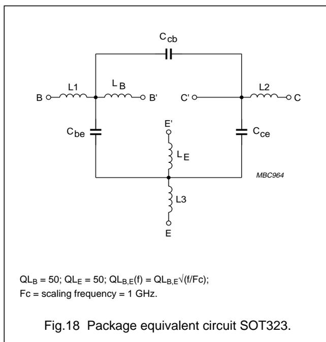
Fig.18 Package equivalent circuit SOT323.
