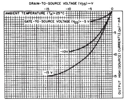
Fig. 11 - Minimum output high (source) current characteristics.
