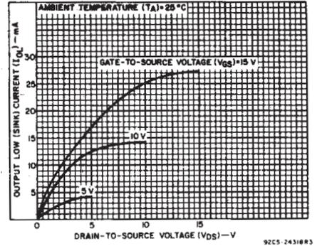
Fig. 7 - Typical output low (sink) current characteristics.
