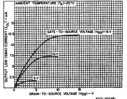
Fig. 8 - Minimum output low (sink) current characteristics.
