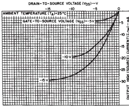
Fig. 10 - Typical output high (source) current characteristics.
