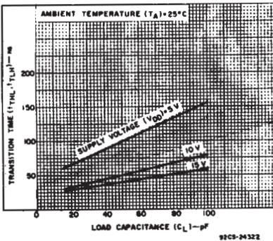
Fig. 9 - Typical transition time vs. load capacitance.
