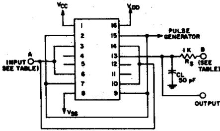
Fig. 12 - Output enable delay times test circuit and waveforms.
