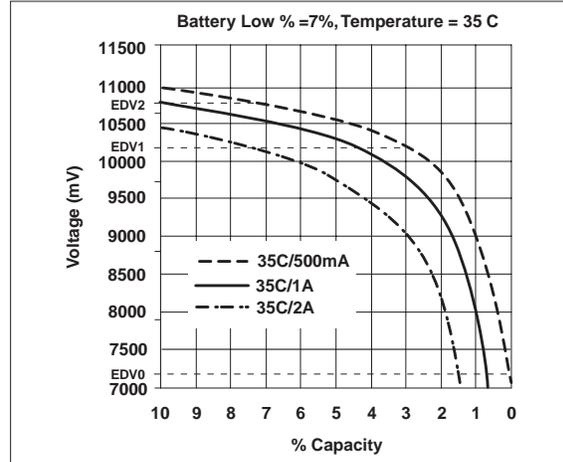
Figure 8. EDV Calculations vs. Capacity for Various Loads
