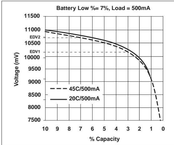
Figure 7. EDV Calculations vs. Capacity for Various Temperatures
