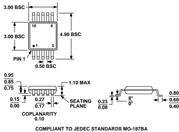
Figure 17. 10-Lead Mini Small Outline Package [MSOP]
