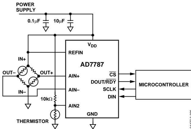
Figure 12. Basic Connection Diagram
