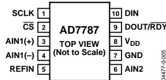
Figure 5. Pin Configuration
