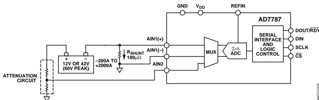
Figure 16. Battery Monitoring
