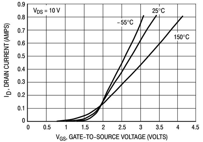
Figure 2. Transfer Characteristics
