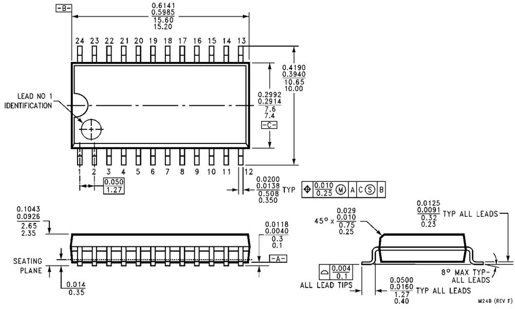
**24-Lead Small Outline Integrated Circuit (SOIC), JEDEC MS-013, 0.300" Wide Body
