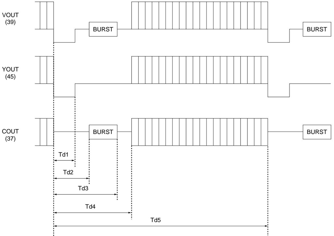
Fig. 20 TV signal timing diagram
