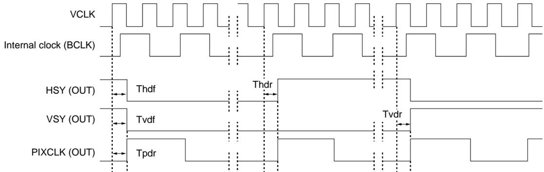
Fig. 16 Output timing with a doubled clock
