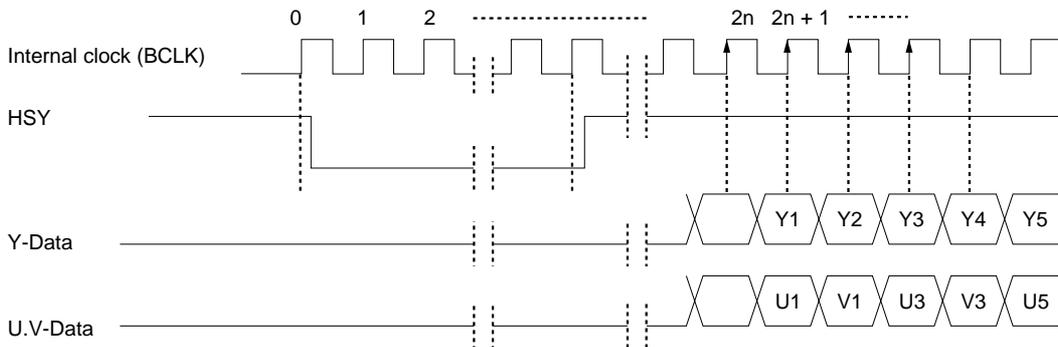
Fig. 26 YUV input timing when TEST[2] = H
