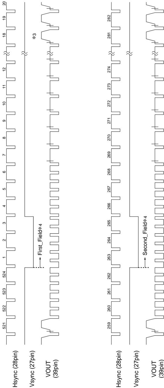
\*3 Indicates a line interval during which video data is output
