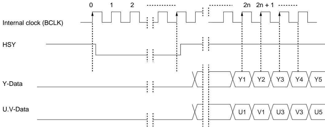
Fig. 25 YUV input timing when TEST[2] = L
