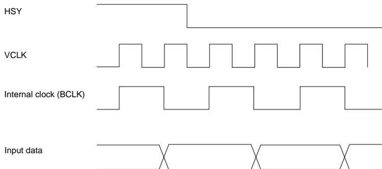
Fig. 3 Illustration of clock timing (CLKSW is LOW)
