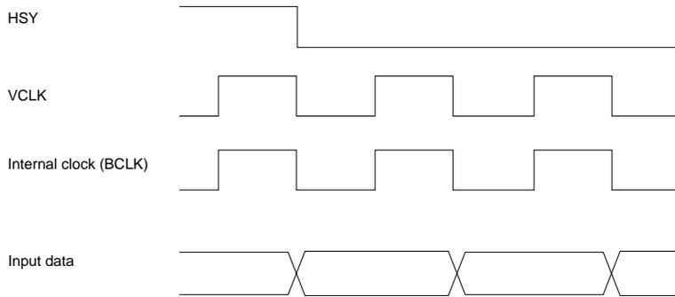
Fig. 4 Illustration of clock timing (CLKSW is HIGH)
