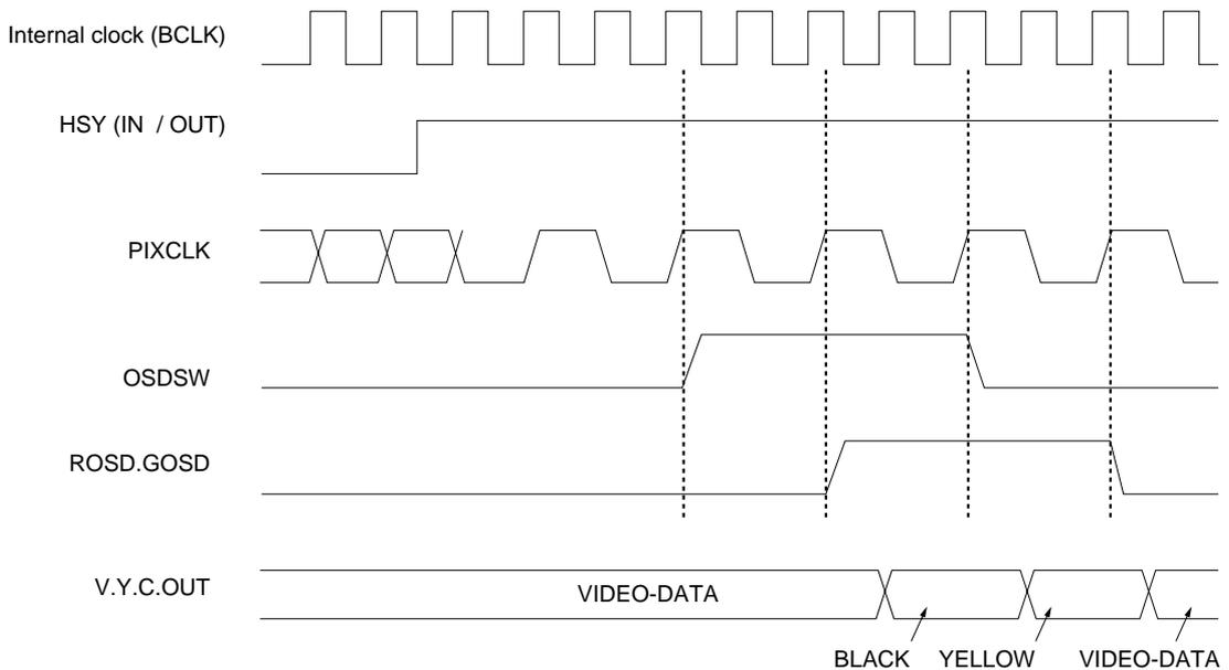
Fig. 15 Clock timing with the OSD function
