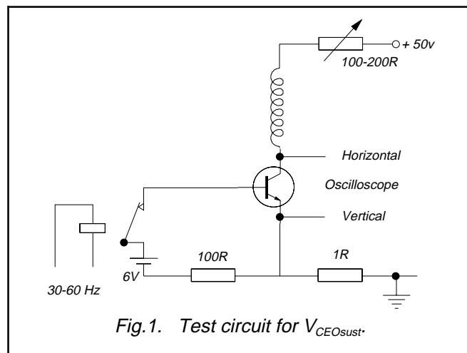
Fig.1. Test circuit for  $V_{CEOus}$ .
