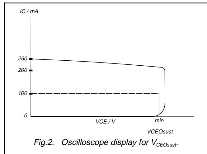
Fig.2. Oscilloscope display for  $V_{CEOus}$ .<sup>1</sup> Measured with half sine-wave voltage (curve tracer).
