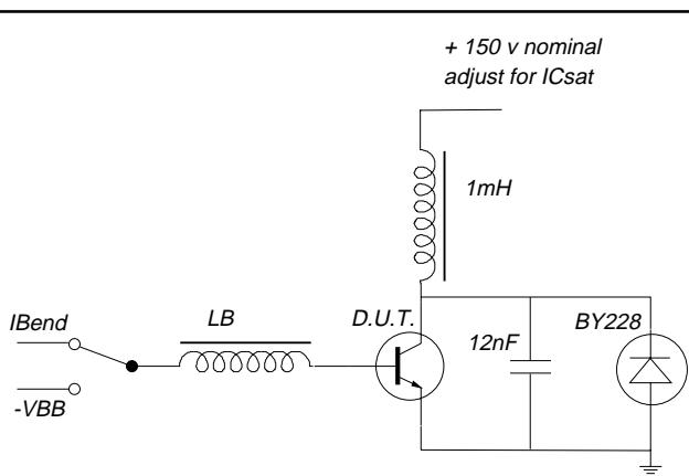
Fig.5. Switching times test circuit.
