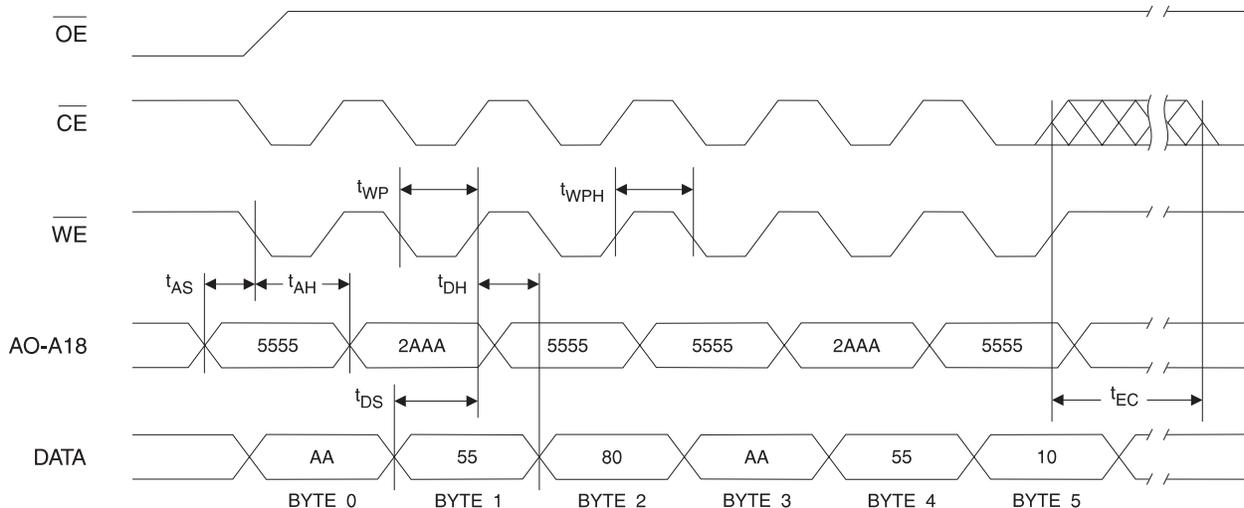
Note:  $\overline{OE}$  must be high only when  $\overline{WE}$  and  $\overline{CE}$  are both low.
