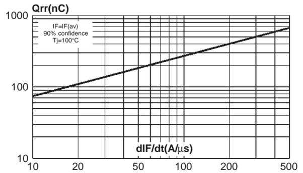
**Fig. 9:** Recovery current versus  $dI_F/dt$  (per diode).
