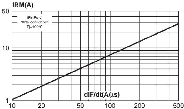
**Fig. 10:** Transient peak forward versus  $dI_F/dt$  (per diode).
