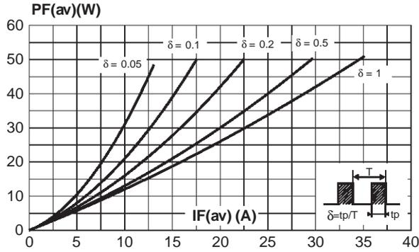
**Fig. 2:** Peak current versus form factor (per diode).
