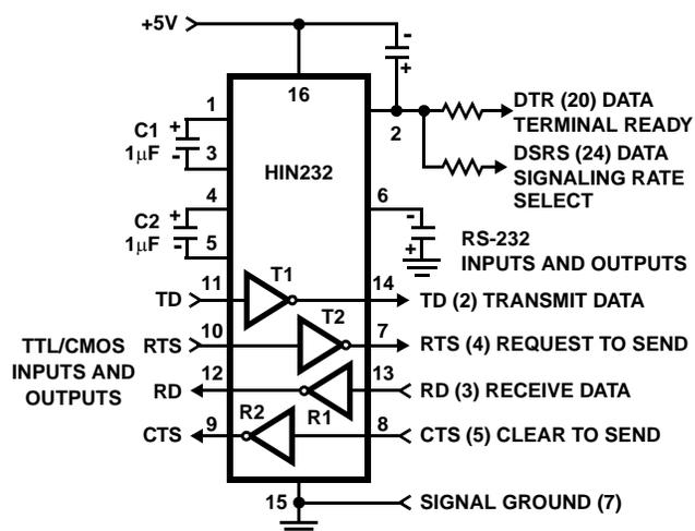
FIGURE 9. SIMPLE DUPLEX RS-232 PORT WITH CTS/RTS HANDSHAKING
