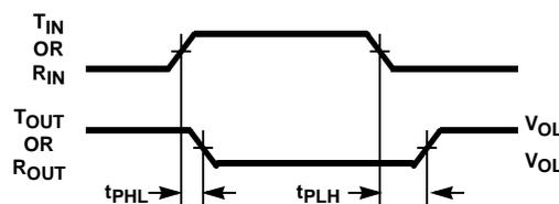
$$\text{Average Propagation Delay} = \frac{t_{PHL} + t_{PLH}}{2}$$
