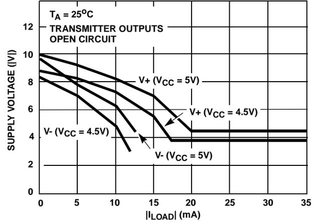
FIGURE 6.  $V_+$ ,  $V_-$  OUTPUT VOLTAGE vs LOAD (HIN232)
