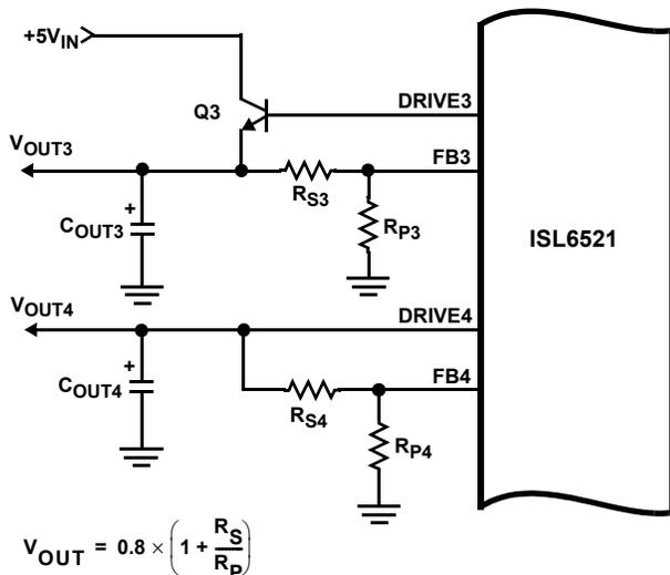
$$V_{OUT} = 0.8 \times \left( 1 + \frac{R_S}{R_P} \right)$$
