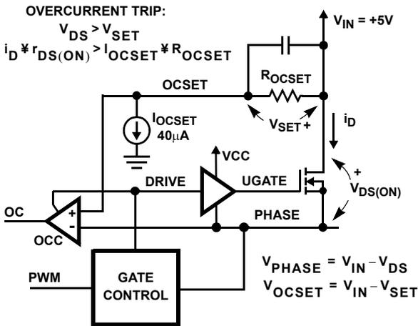
FIGURE 3. OVERCURRENT DETECTION
