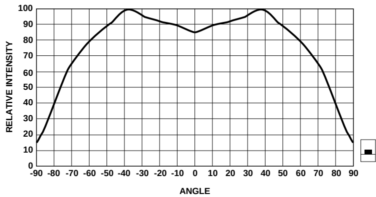
Figure 6. Relative intensity vs. angle for HSMx-C120.
