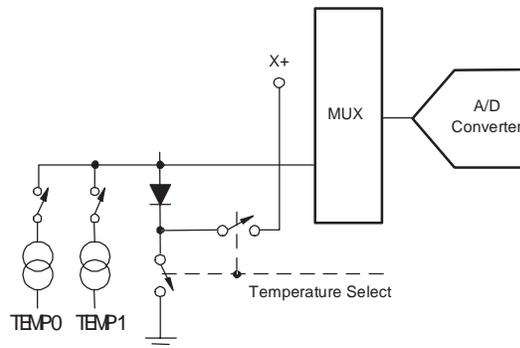
**Figure 14. Functional Block Diagram of Temperature Measurement Mode**
