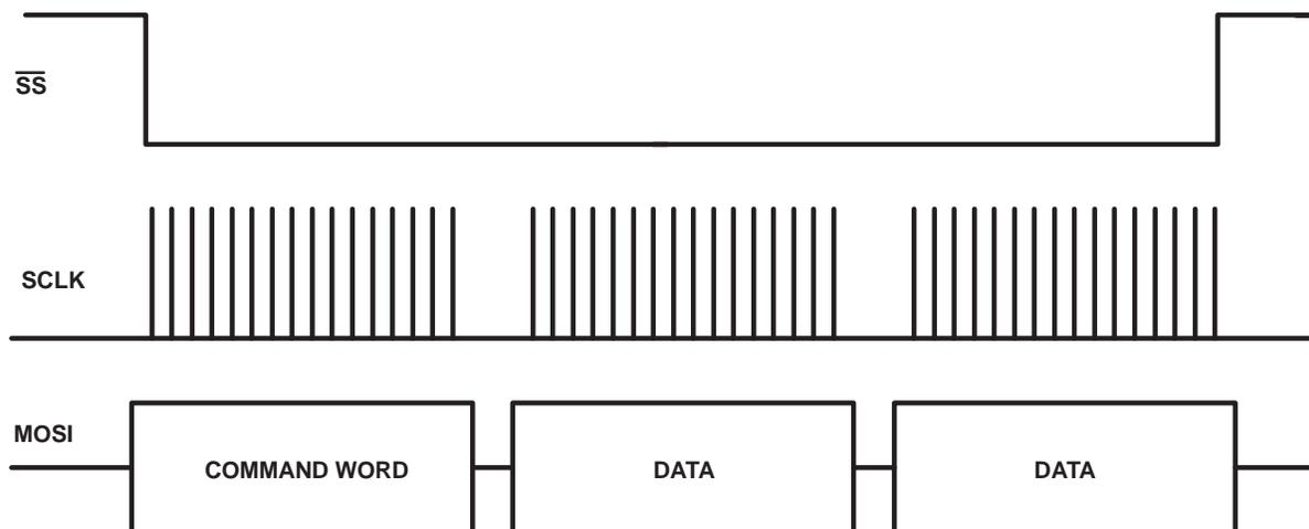
**Figure 24. Write Operation for TSC2102 SPI Interface**
