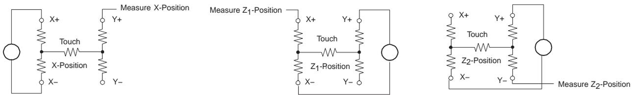
**Figure 11. Pressure Measurement**
