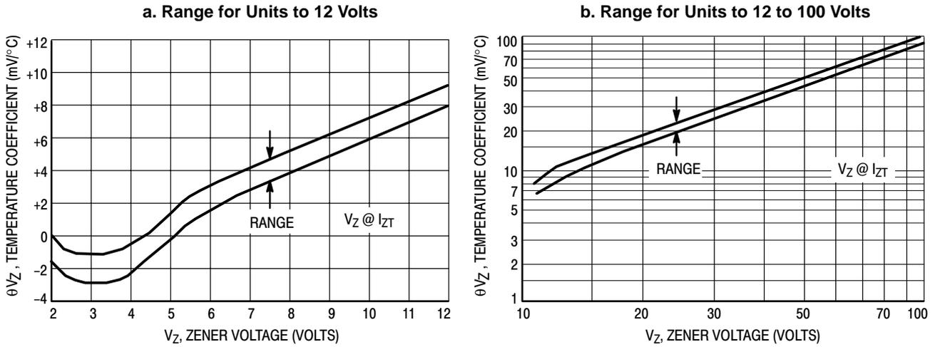
**Figure 2. Temperature Coefficients**
