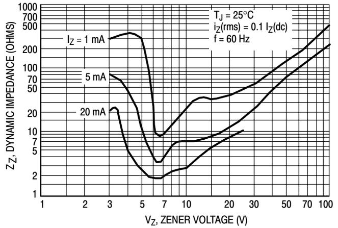
**Figure 7. Effect of Zener Voltage on Zener Impedance**
