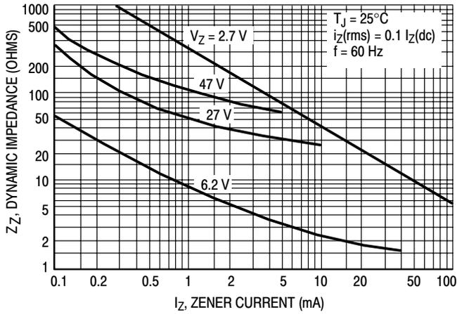
**Figure 6. Effect of Zener Current on Zener Impedance**
