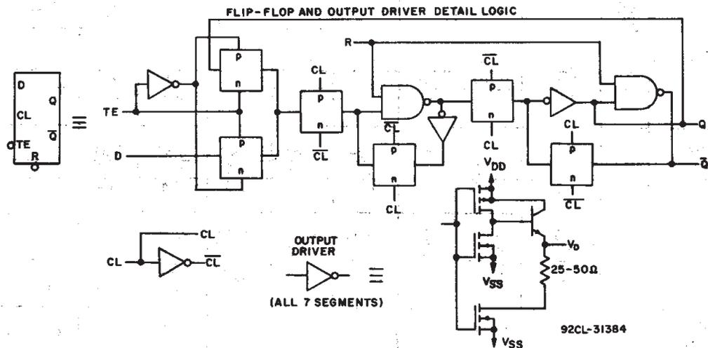
Fig. 2 - Logic diagram with flip-flop and output-driver details.
