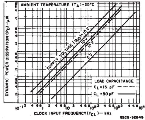
Fig. 10 - Typical dynamic power dissipation vs. frequency.
