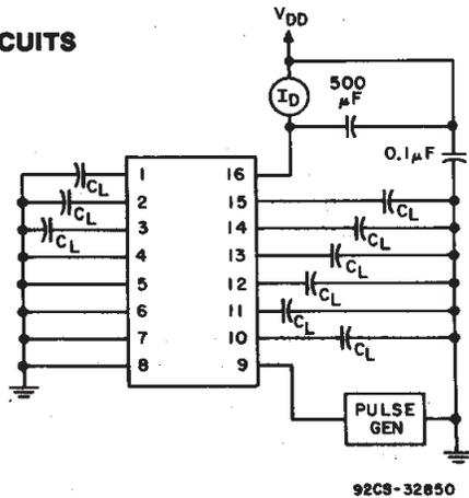
Fig. 11 - Dynamic power dissipation test circuit.
