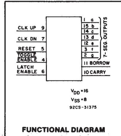
■ CD40110B is a dual-clocked up/down counter with a special preconditioning circuit that allows the counter to be clocked, via positive going inputs, up or down regardless of the state or timing (within 100 ns typ.) of the other clock line.
