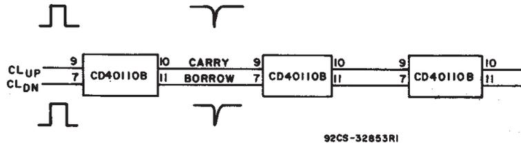
Fig. 15 - Cascading diagram.
