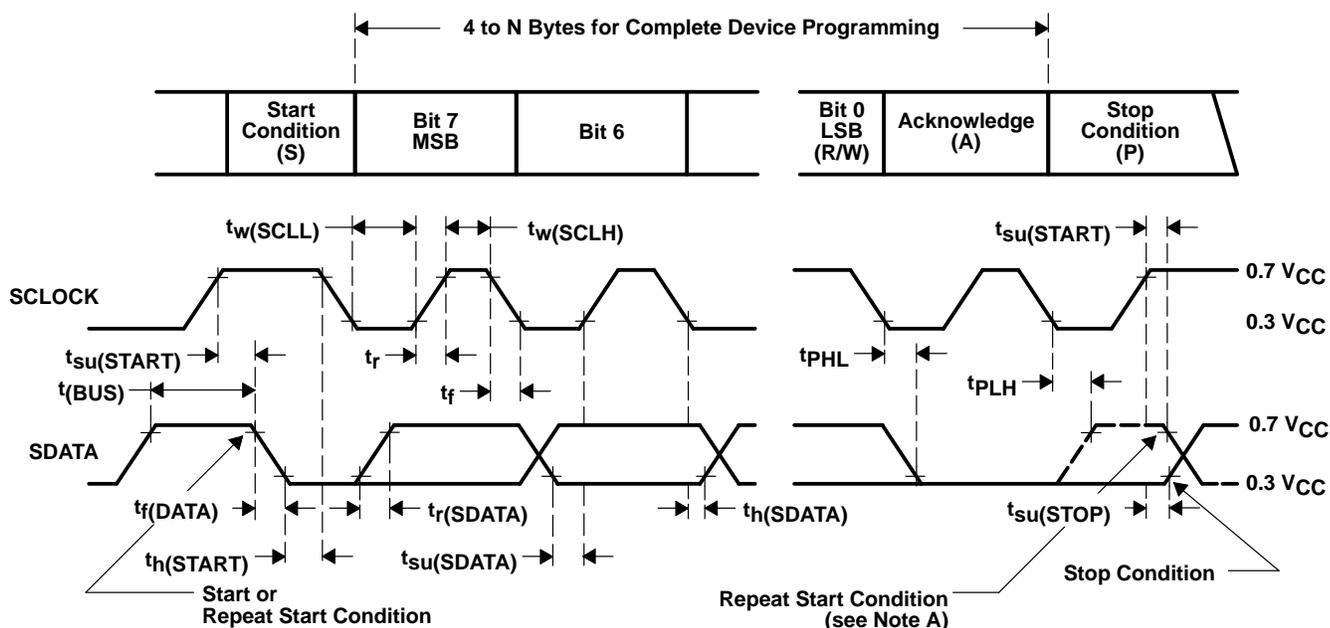
NOTE A: The repeat start condition is supported, but not clock stretching.
