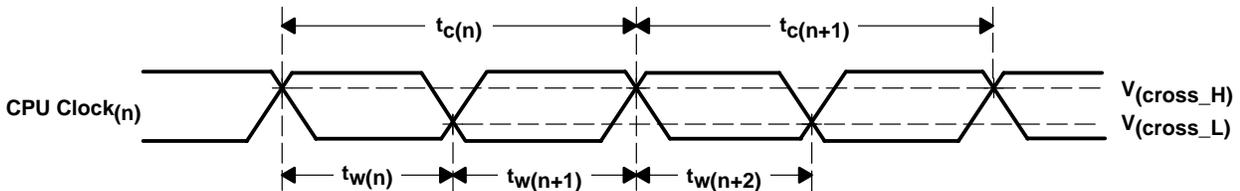
Cycle-to-Cycle Jitter  $t_{jit(cc)} = |t_{c(n)} - t_{c(n+1)}|$  |  $n > 2 \times 10^3$
