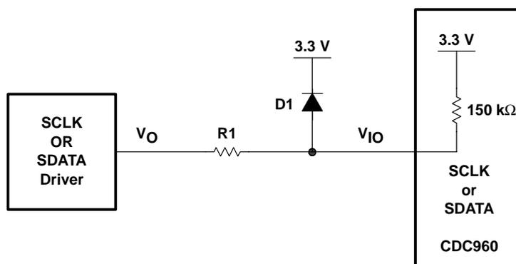
**Figure 2. SCLK SDATA Connection to 5-V SMBus Using Clamping Diode to  $V_{DD}$**
