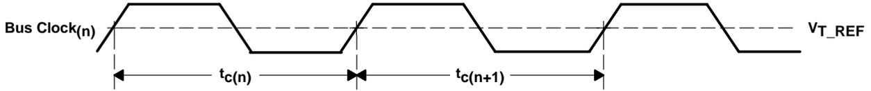
Cycle-to-Cycle Jitter  $t_{jit(cc)} = |t_{c(n)} - t_{c(n+1)}|$  |  $n > 2 \times 10^3$
