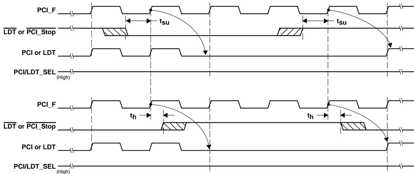
NOTE: Assertion and deassertion of  $\overline{\text{PCI\_STOP}}$  or  $\overline{\text{LDT\_STOP}}$  maintain signals duty cycle.
