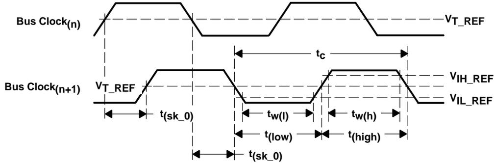
$$t(sk_p) = |t_w(l) - t_w(h)| \qquad \text{Duty Cycle} = \frac{t(low \text{ or } high)}{t_c} \times 100$$
