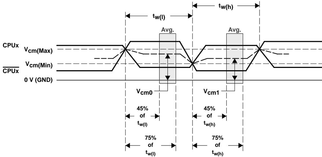
$V_{cm0}$  is calculated from the average of  $V_{ocm}$  within 45%–75% (region without switching noise) of the pulse while CPUx is in the LOW state.
