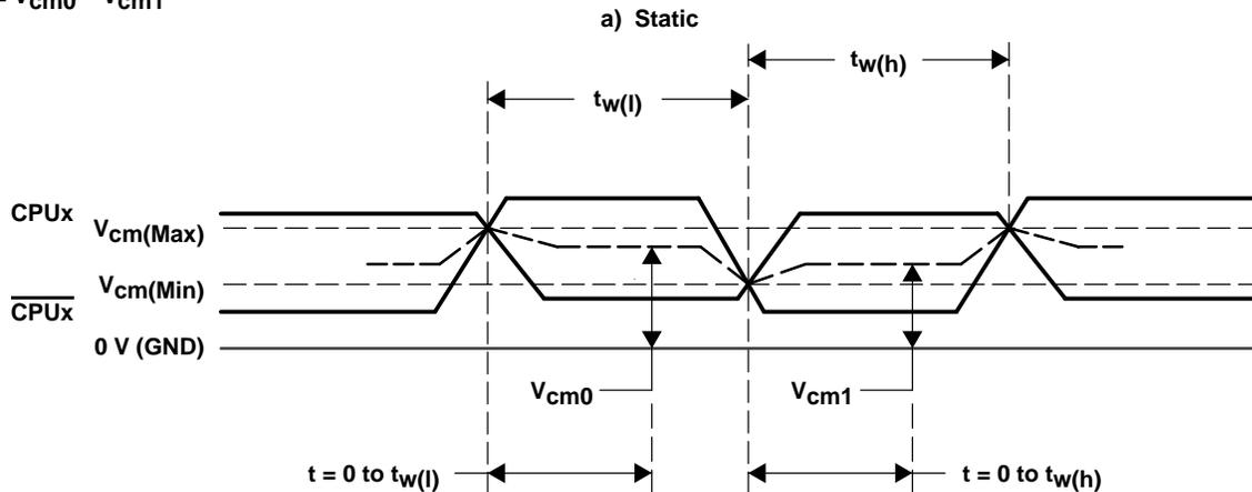
$$\Delta V_{ocm}(t) = \text{MAX}(V_{cm0}(t)) - \text{MIN}(V_{cm1}(t)) \text{ and}$$
