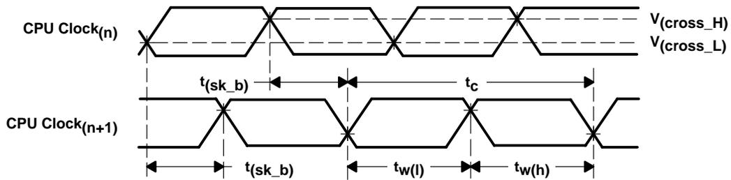
$$\text{Duty Cycle} = \frac{t_w(\text{Low or High})}{t_c} \times 100$$
