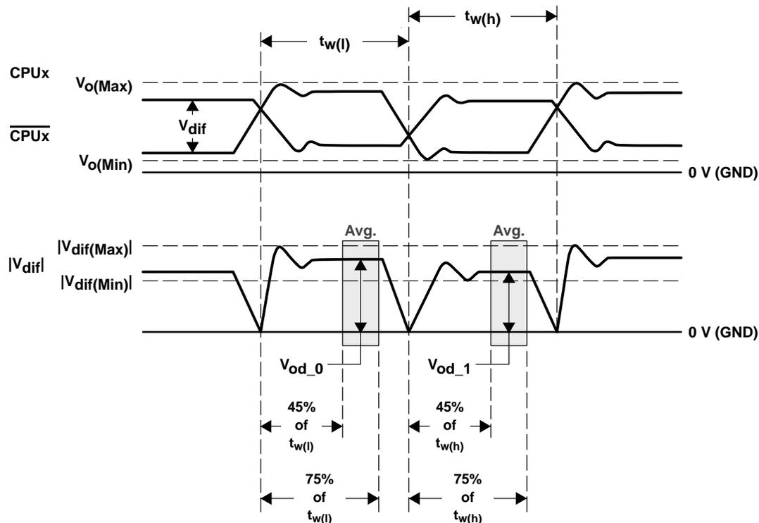
$V_{od\_0}$  is calculated from the average of  $V_{od}$  within 45%–75% (region without switching noise) of the pulse while CPUx is in the LOW state.
