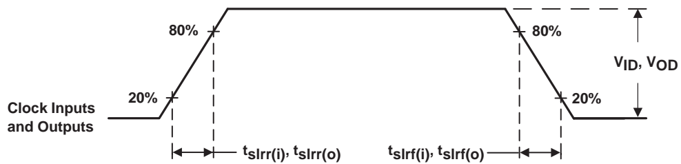
Figure 8. Input and Output Slew Rates
