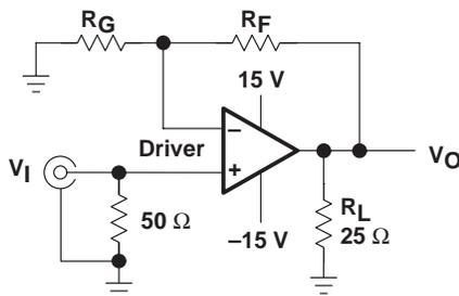
Figure 3. Driver Test Circuit, Gain =  $1 + (R_F/R_G)$
