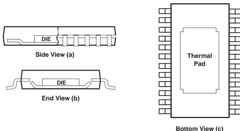
NOTE A: The thermal pad is electrically isolated from all terminals in the package.
