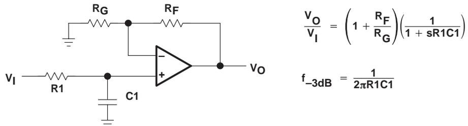
**Figure 61. Single-Pole Low-Pass Filter**
