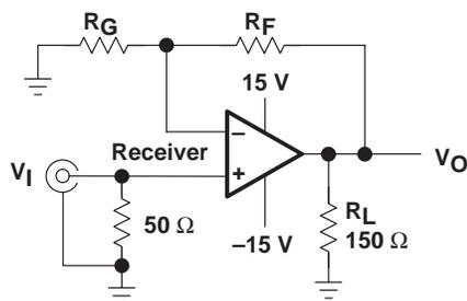
Figure 4. Receiver Test Circuit, Gain =  $1 + (R_F/R_G)$
