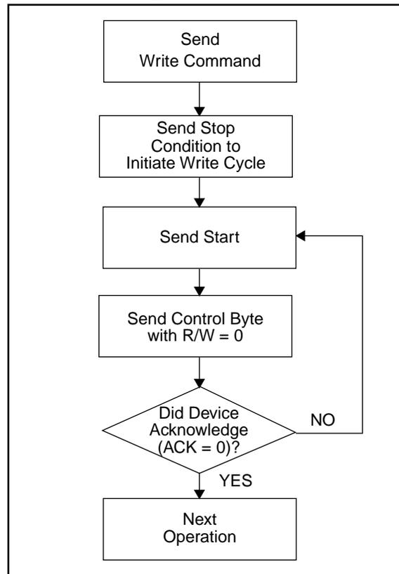
**FIGURE 6-5: BYTE WRITE**
