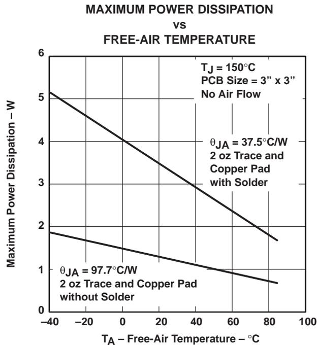
Figure 59. Maximum Power Dissipation vs Free-Air Temperature
