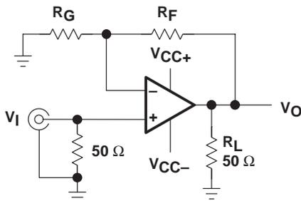
Figure 2. Test Circuit, Gain =  $1 + (R_F/R_G)$
