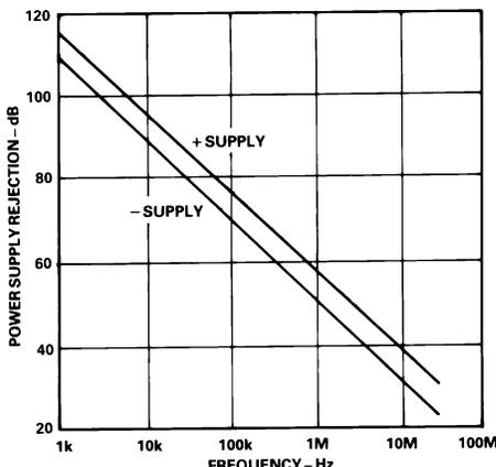
Figure 20. Power Supply Rejection vs. Frequency (AD849)
