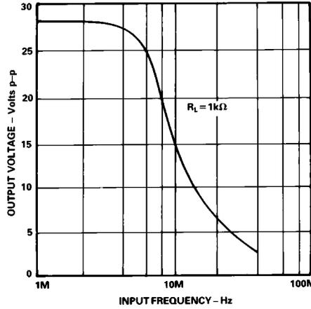
Figure 5. Large Signal Frequency Response (AD848 and AD849)
