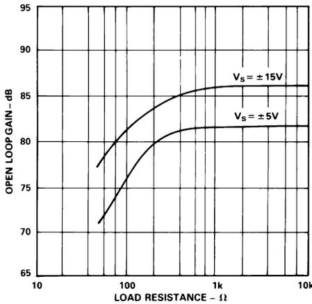
Figure 7. Open Loop Gain vs. Load Resistance (AD848)
