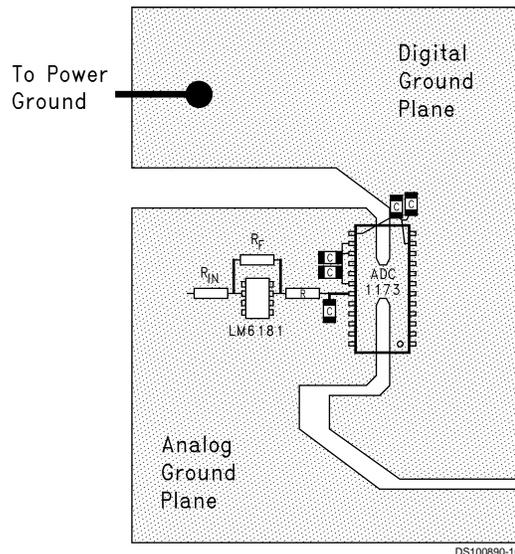
**FIGURE 6. Layout example showing separate analog and digital ground planes connected below the ADC1173.**
