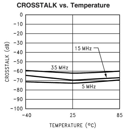
**Typical Performance Characteristics**  $V_A = V_D = 3.3V$ ,  $V_{DR} = 2.5V$ ,  $f_{CLK} = 40\text{ MHz}$ ,  $f_{IN} = 10.4\text{ MHz}$ , unless otherwise specified (Continued)
