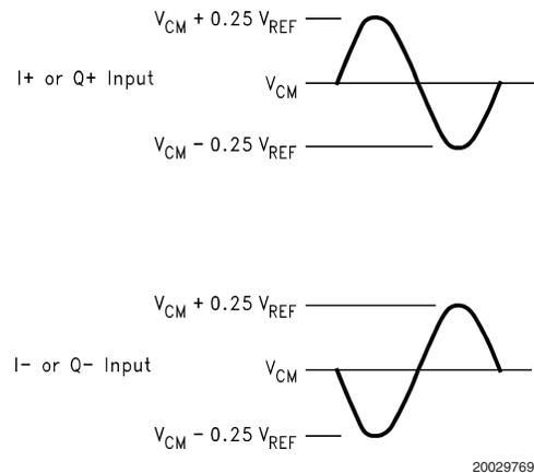
**FIGURE 2. The ADC10D040 is designed for use with differential signals of  $1.4 V_{P-P}$  with a common mode voltage of 1.5V. The signal swing should not cause any pin to experience a swing more than 300 mV beyond the supply rails.**
