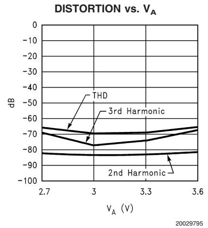
**Typical Performance Characteristics**  $V_A = V_D = 3.3V$ ,  $V_{DR} = 2.5V$ ,  $f_{CLK} = 40$  MHz,  $f_{IN} = 10.4$  MHz, unless otherwise specified (Continued)
