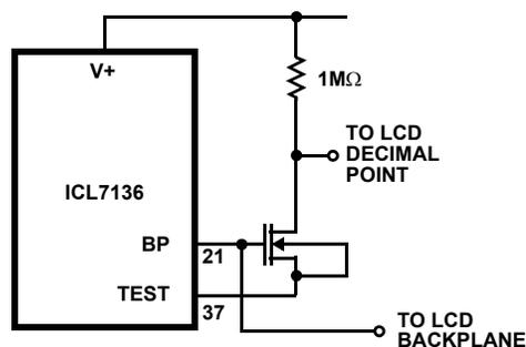
FIGURE 4. SIMPLE INVERTER FOR FIXED DECIMAL POINT
