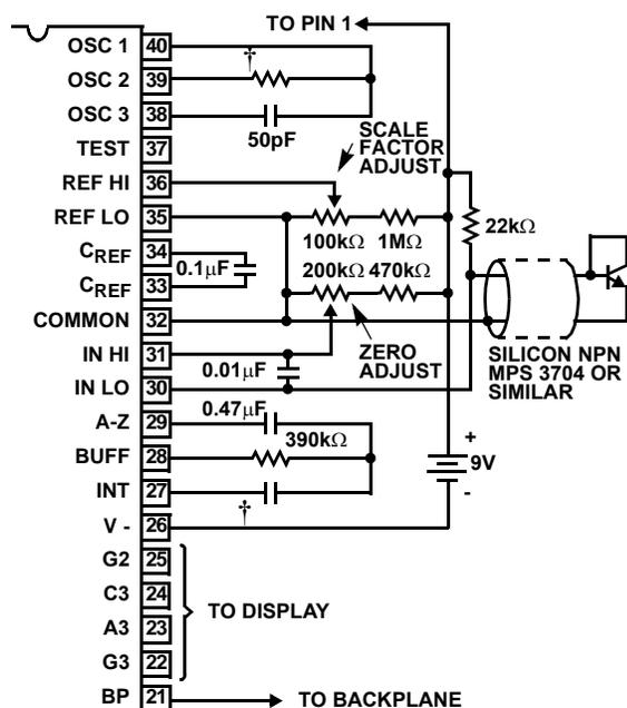
A silicon diode-connected transistor has a temperature coefficient of about  $-2\text{mV}/^\circ\text{C}$ . Calibration is achieved by placing the sensing transistor in ice water and adjusting the zeroing potentiometer for a 000.0 reading. The sensor should then be placed in boiling water and the scale-factor potentiometer adjusted for a 100.0 reading.
