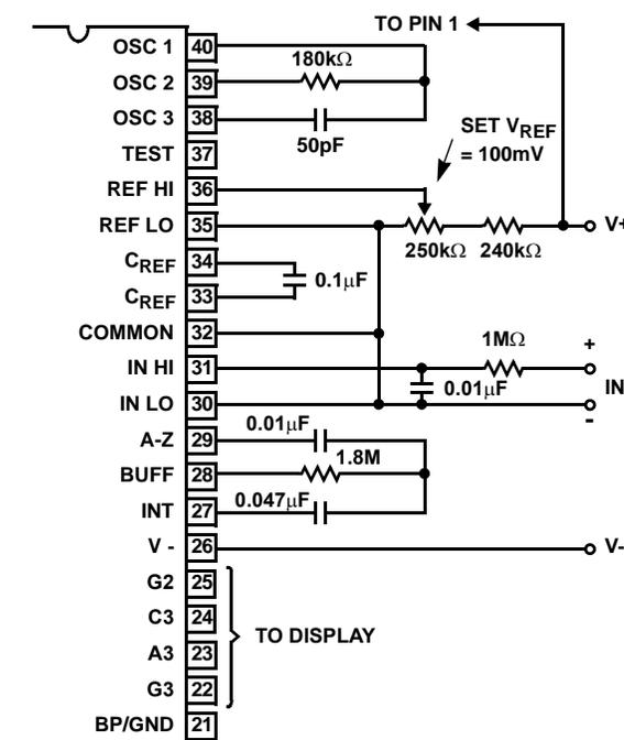
FIGURE 9. RECOMMENDED COMPONENT VALUES FOR 2V FULL SCALE
