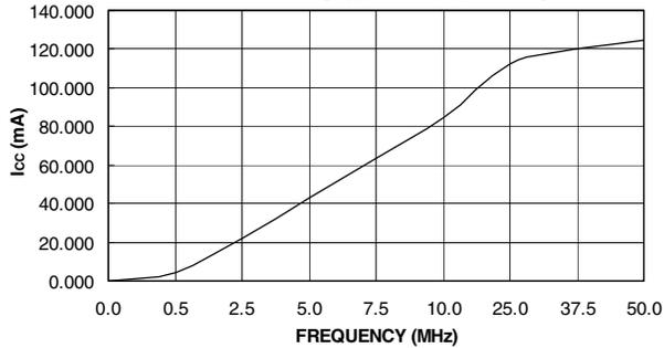
**ATF22V10CQZ SUPPLY CURRENT vs. INPUT FREQUENCY ( $V_{CC} = 5\text{V}$ ,  $T_A = 25^\circ\text{C}$ )**
