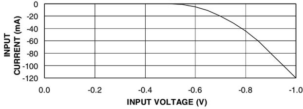
**ATF22V10CZ/CQZ INPUT CURRENT VS INPUT VOLTAGE ( $V_{CC} = 5V$ ,  $T_A = 25^\circ C$ )**
