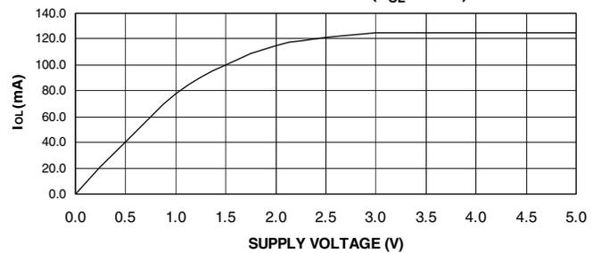
**ATF22V10CZ/CQZ INPUT CLAMP CURRENT VS INPUT VOLTAGE ( $V_{CC} = 5V$ ,  $T_A = 35^\circ C$ )**
