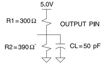
Note: Similar competitors devices are specified with slightly different loads. These load differences may affect output signals' delay and slew rate. Atmel devices are tested with sufficient margins to meet compatible device specification conditions.
