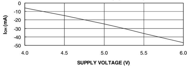
**ATF22V10CZ/CQZ OUTPUT SOURCE CURRENT vs. OUTPUT VOLTAGE ( $V_{CC} = 5\text{V}$ ,  $T_A = 25^\circ\text{C}$ )**
