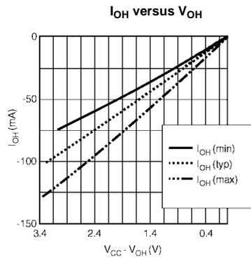
FIGURE 1. Characteristics for Output - Pull Up Drive
