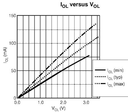
FIGURE 2. Characteristics for Output - Pull Down Driver
