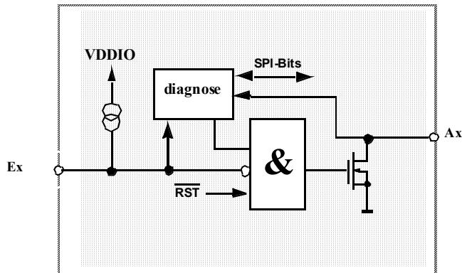
The transmit-function has to be enabled via SPI soft reset after an active RST (low). The open-drain outputs are current-limited, in addition the output voltage on Ax ( $x=1;2$ ) is monitored for plausibility. If the voltage at Ax still exceeds a certain defined threshold after switch on the output transistor and after a predefined time  $t_{off}$ , a short-circuit to battery is detected and the stage is turned off.
