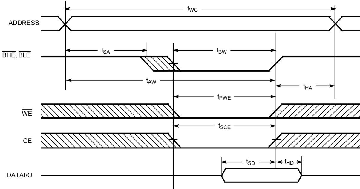
Write Cycle No. 3 ( $\overline{\text{WE}}$  Controlled,  $\overline{\text{OE}}$  HIGH During Write)<sup>[16, 17]</sup>
