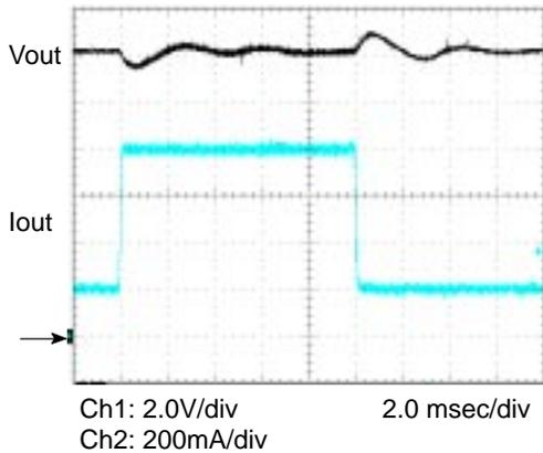
Figure 14. Load Regulation 120V
