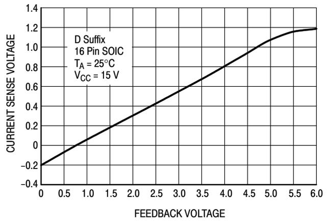
Figure 10. Feedback Voltage versus Current Sense Voltage
