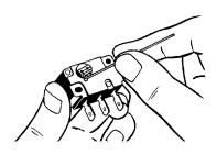
Push the lever down in the direction of the groove in the rotary disc.
