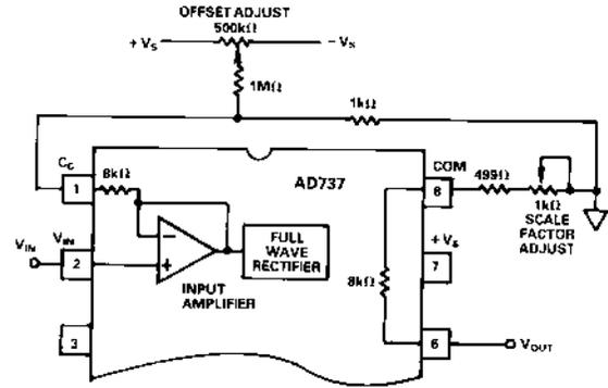
Figure 23. DC Coupled  $V_{OS}$  and Scale Factor Trims
