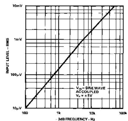
Figure 9. 23 dB Frequency vs. RMS Input Level (Pin 2)
