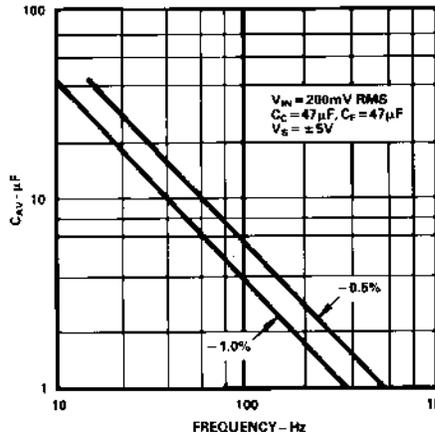
Figure 11.  $C_{AV}$  vs. Frequency for Specified Averaging Error
