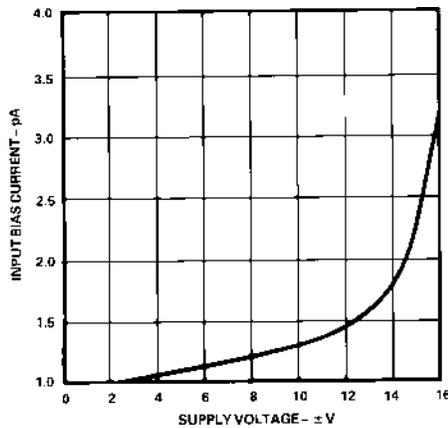
Figure 13. Pin 2 Input Bias Current vs. Supply Voltage
