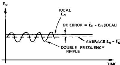
Figure 18. Output Waveform for Sine-Wave Input Voltage
