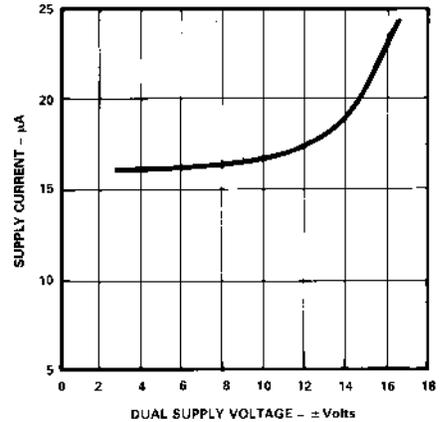
Figure 3. Power Down Current vs. Supply Voltage
