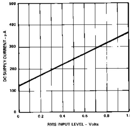
Figure 8. DC Supply Current vs. RMS Input Level
