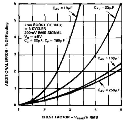
Figure 6. Additional Error vs. Crest Factor vs.  $C_{AV}$
