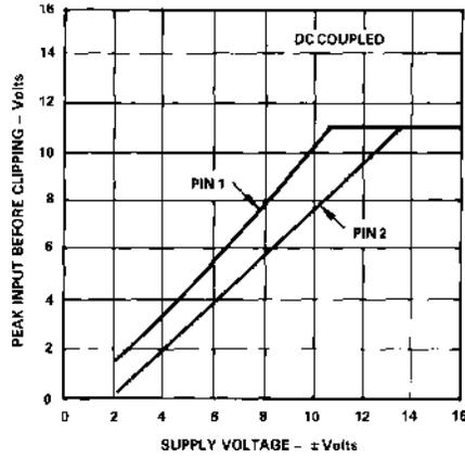
Figure 2. Maximum Input Level vs. Supply Voltage
