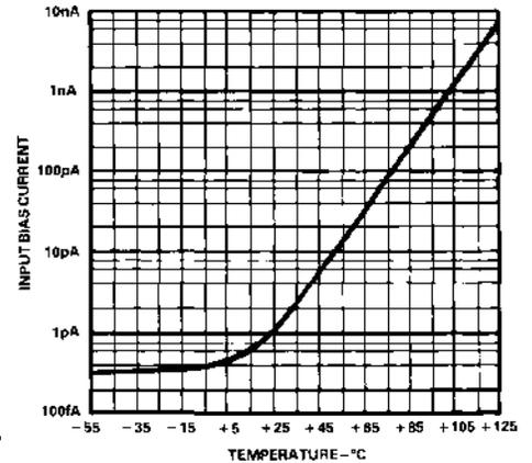
Figure 15. Pin 2 Input Bias Current vs. Temperature
