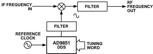
Figure 3. Frequency/Phase-Agile Local Oscillator for Frequency Mixing/Multiplying
