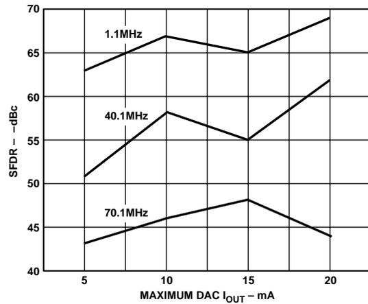
Figure 42. Effect of DAC maximum output current on wideband (0 to 72 MHz) SFDR at three representative DAC output frequencies: 1.1 MHz, 40.1 MHz and 70.1 MHz.  $V_S = +5V$ , 180 MHz system clock ( $6\times REFCLK$  Multiplier disabled). Currents are set using appropriate values of  $R_{SET}$ .
