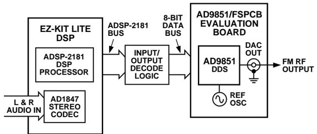
Figure 6. High Quality, All-Digital RF Frequency Modulation
