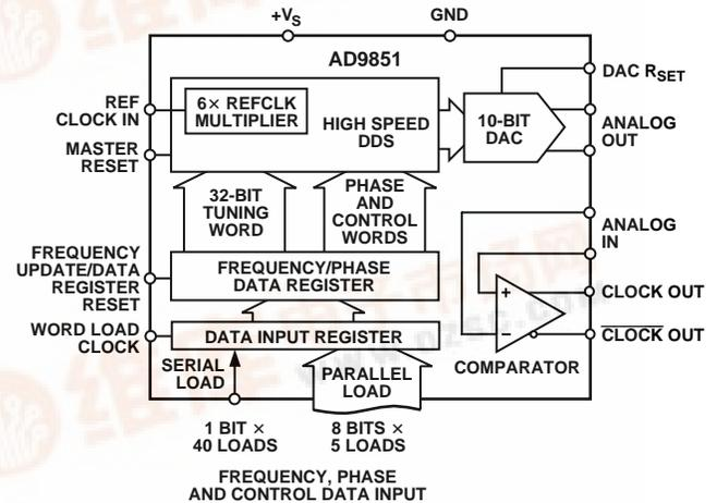
The AD9851 contains an internal high speed comparator that can be configured to accept the (externally) filtered output of the DAC to generate a low jitter output pulse.
