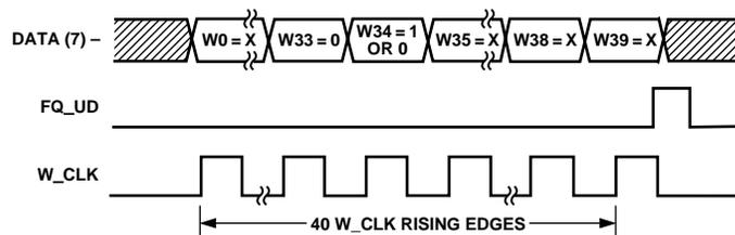
Figure 20. Serial-Load Power-Down/Power-Up Sequence
