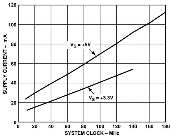
Figure 41. Supply current variation with system clock frequency.
