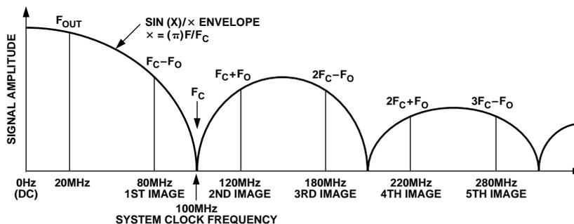
Figure 12. Output Spectrum of a Sampled Sin(X)/X Signal
