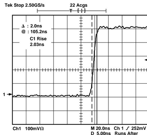
Figure 38. Comparator Rise Time, 15 pF Load
