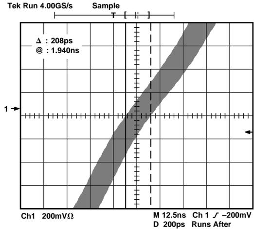
Figure 32. Typical CMOS comparator p-p output jitter with the AD9851 configured as a clock generator, DDS  $f_{OUT} = 10.1$  MHz,  $V_S = +5$  V, system clock = 180 MHz, 70 MHz LPF. Graph details the center portion of a rising edge with scope in delayed trigger mode, 200 ps/div. Cursors show 208 ps p-p jitter.
