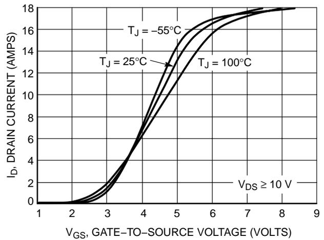
**Figure 2. Transfer Characteristics**
