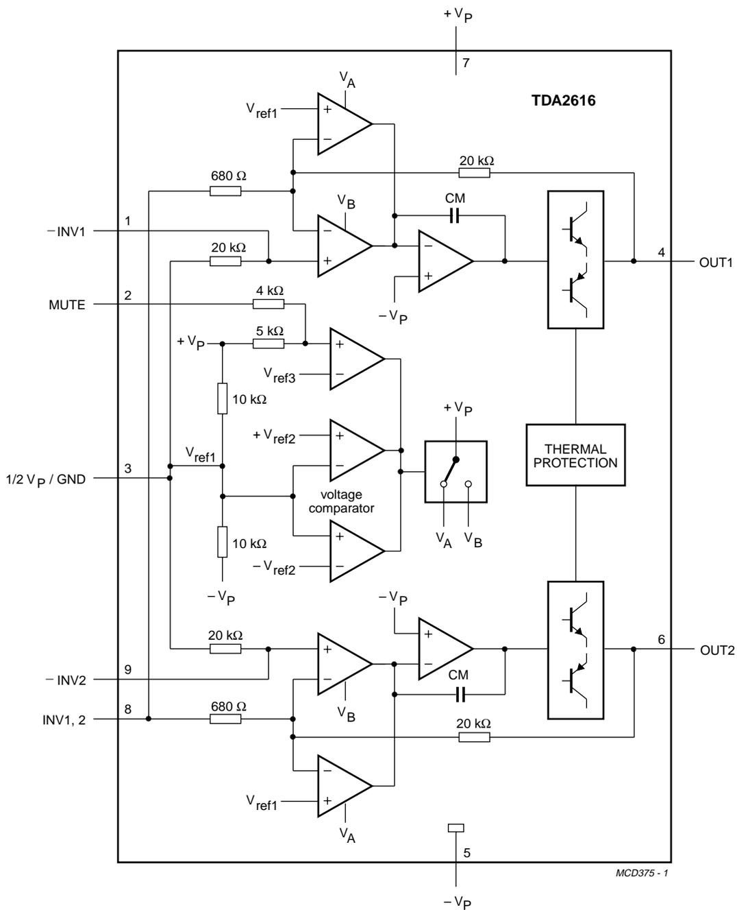
Fig.1 Block diagram.
