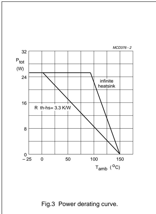
Fig.3 Power derating curve.
