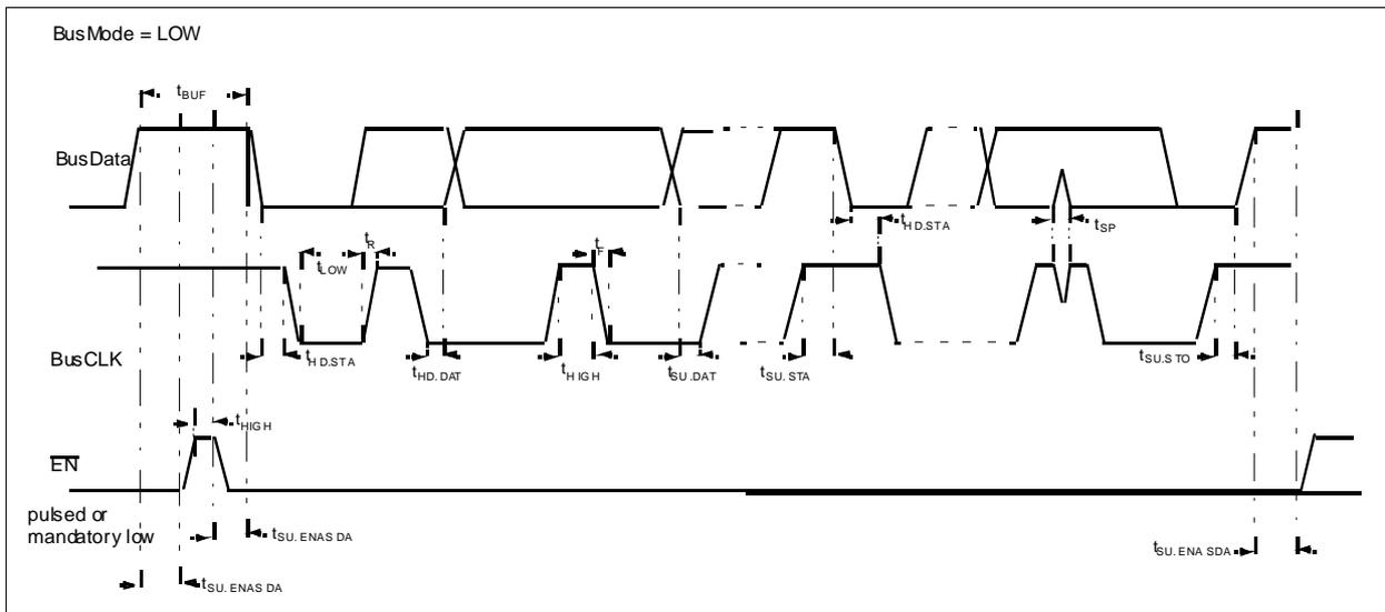
Figure 4-1 I<sup>2</sup>C Bus Timing
