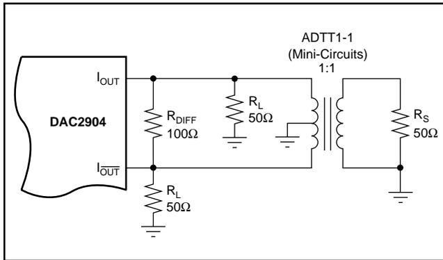
FIGURE 3. Differential Output Configuration Using an RF Transformer.
