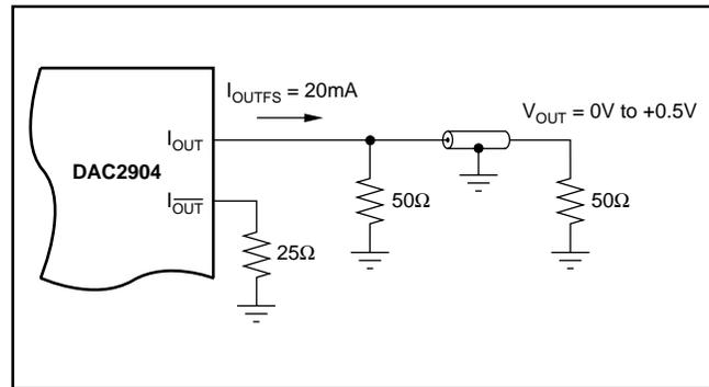
FIGURE 6. Driving a Doubly Terminated  $50\Omega$  Cable Directly.
