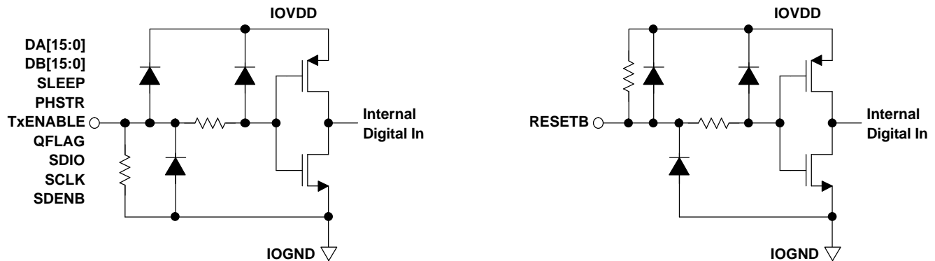
Figure 42. CMOS/TTL Digital Equivalent Input
