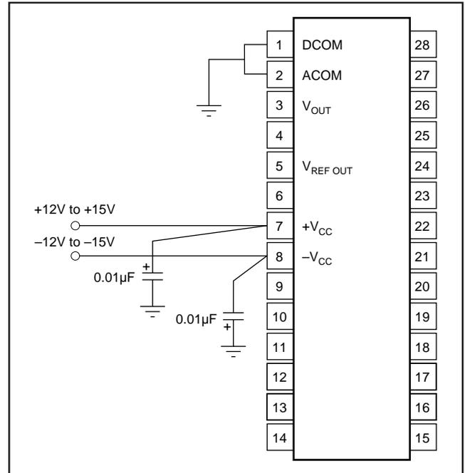
FIGURE 4. Power Supply Connections.
