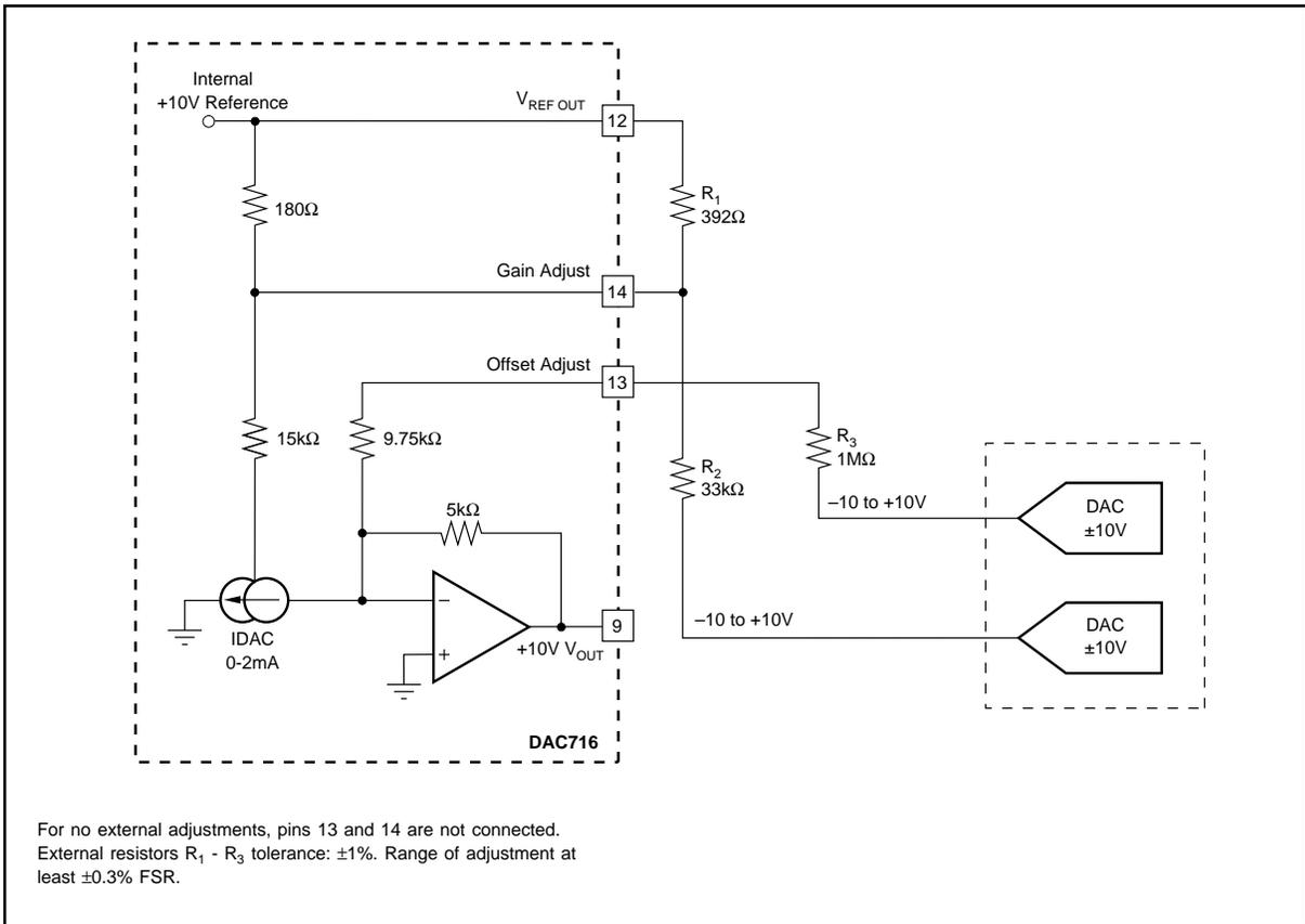
FIGURE 7. Gain and Offset Adjustment Using D/A Converters.
