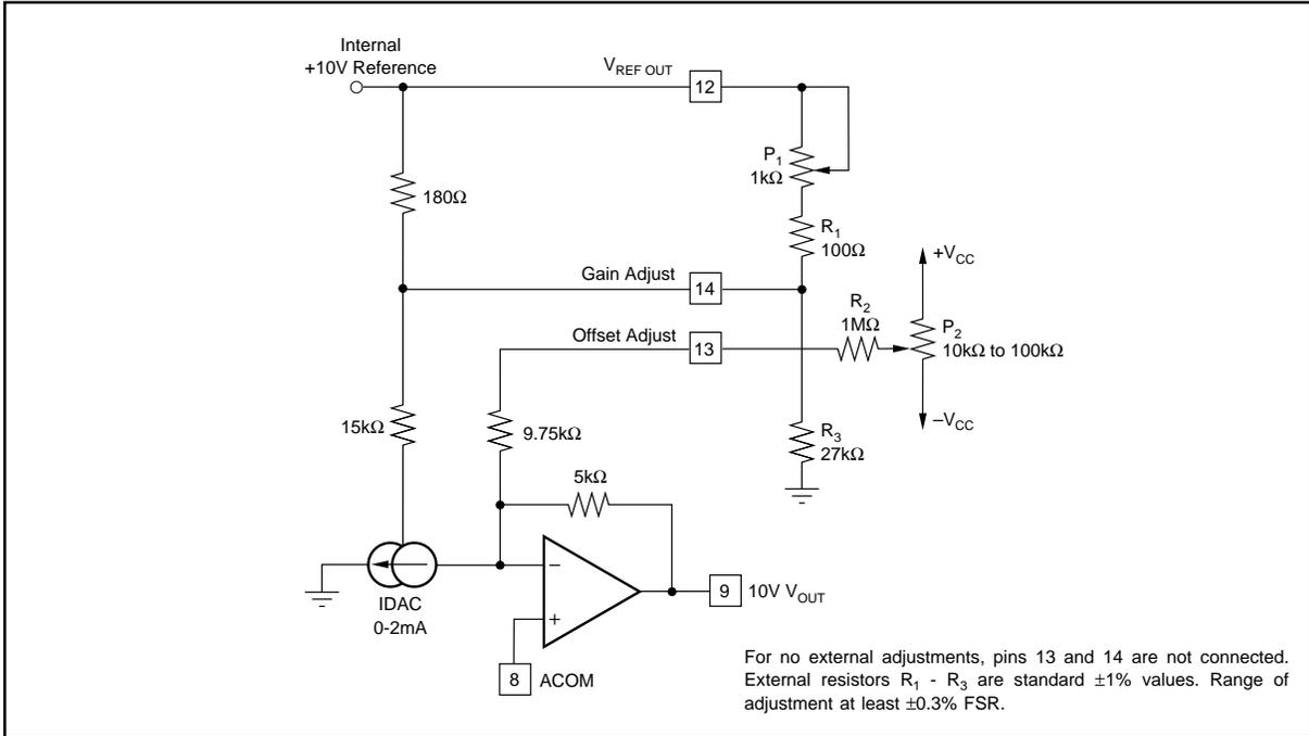
FIGURE 6. Manual Offset and Gain Adjust Circuits.
