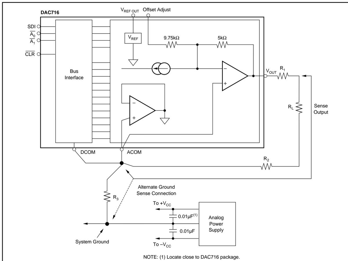
FIGURE 5. System Ground Considerations for High-Resolution D/A Converters.
