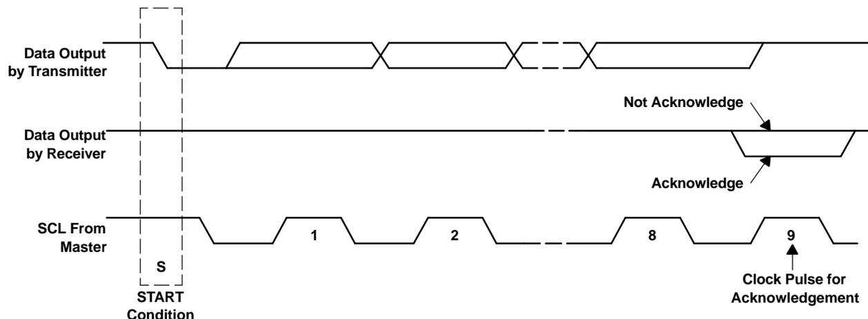
**Figure 42. Acknowledge on the I<sup>2</sup>C Bus**
