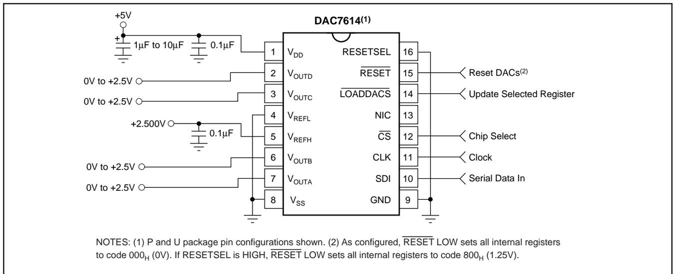
FIGURE 1. Basic Single-Supply Operation of the DAC7614.
