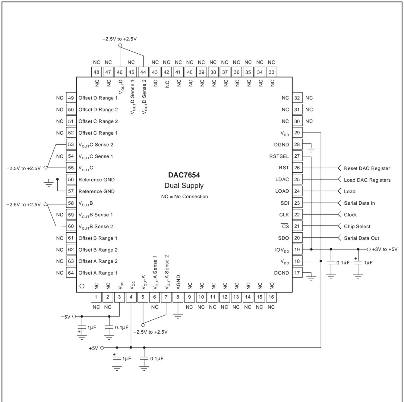
**Figure 55. Basic Dual-Supply Operation of the DAC7654**
