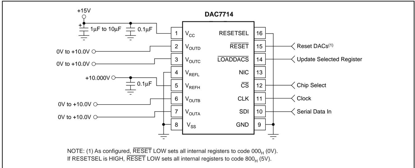
FIGURE 2. Basic Single-Supply Operation of the DAC7714.
