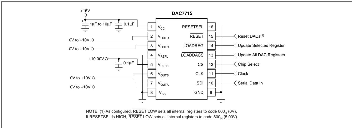
FIGURE 2. Basic Single-Supply Operation of the DAC7715.
