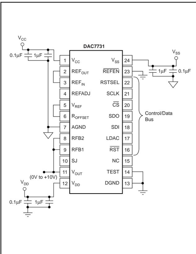
FIGURE 2. Basic Operation:  $V_{OUT} = 0V$  to +10V.
