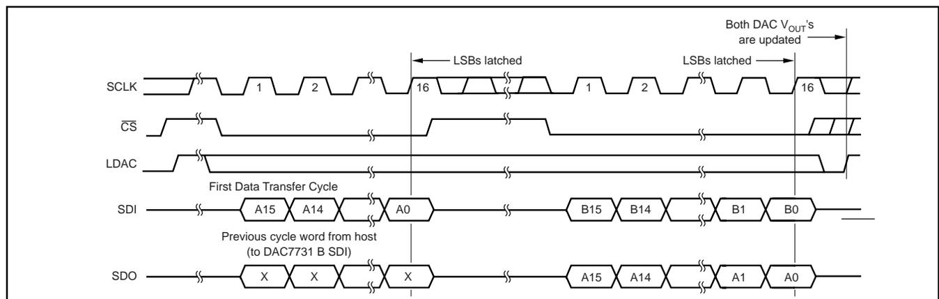
FIGURE 8. DAC7731 Daisy-Chain Timing for Figure 7.
