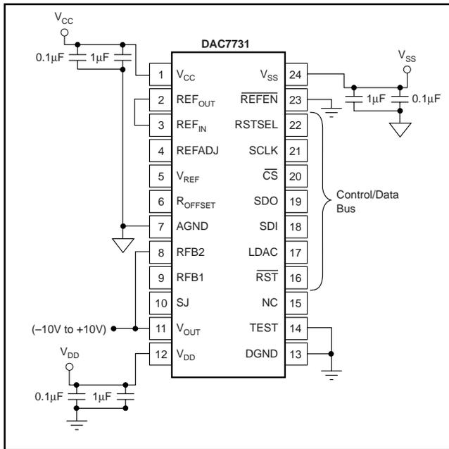
FIGURE 4. Basic Operation:  $V_{OUT} = -10V$  to  $+10V$ .
