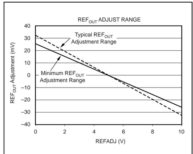
FIGURE 13. Internal Reference Adjustment Transfer Characteristic.
