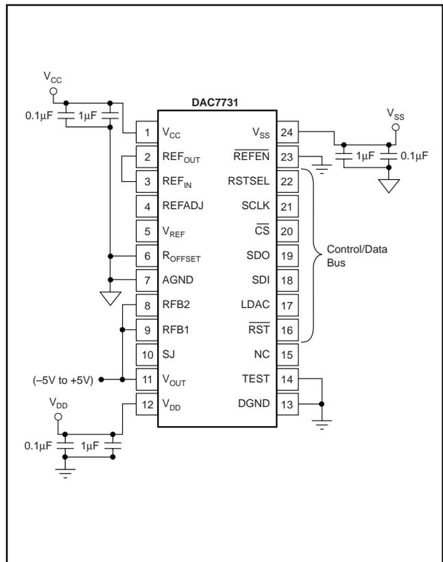
FIGURE 3. Basic Operation:  $V_{OUT} = -5V$  to +5V.
