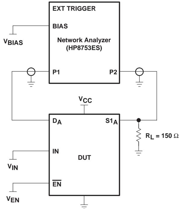
Figure 7. Test Circuit for Frequency Response (BW)
