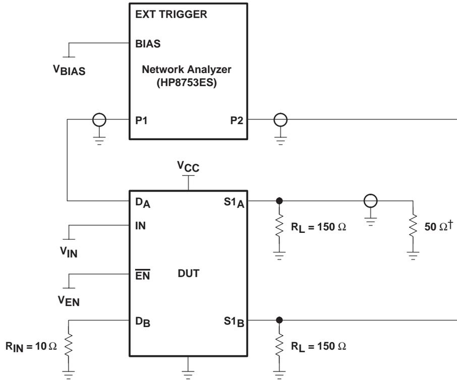
† A 50-Ω termination resistor is needed for the network analyzer.
